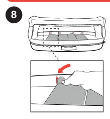
8. Locate the 4 Divider Panels underneath the Changer. Each Divider Panel has 2 tabs on each end. Stand the Divider Panel up and insert both tabs into the slot on the bottom lip of the Changer. Repeat for the other 3 Divider Panels
