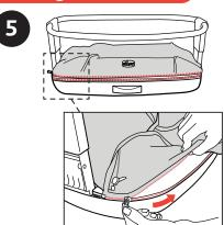
5. Locate the bottom zipper section on the Changer/Parent Organizer Fabric and line it up with the zipper section on the Bassinet Floor. Connect both sections and zip the sections together. Repeat for the other side.
