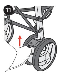
11. To unlock the braking system, push each one of the two levers located at the center of the rear wheel units in an upward direction.
