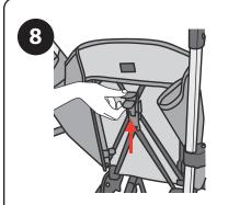
8. To recline the Backrest, squeeze together both levers and pull down on the Backrest. To adjust the Backrest into an upright position, push up on the Backrest until it locks into the desired position.
