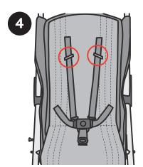
4. This stroller has a five-point safety harness featuring two shoulder straps, two adjustment holes, a waist strap and a crotch strap with buckle.
