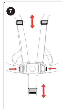
7. The length of the Shoulder Straps and Crotch Strap can be adjusted by pulling on the adjustment buckles to tighten or loosen.
