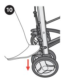
10. To apply the brakes, push on each of the two levers located at the center of the rear wheel units in a downward direction.
