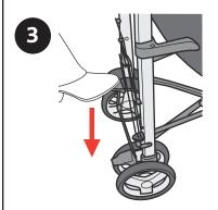
3. Push the rear locking mechanism downward with your foot. Ensure that the stroller is open and locked in the correct position.
