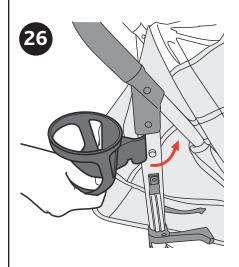
26. Attach the cupholder to the right leg of the stroller just above the carrying handle.
