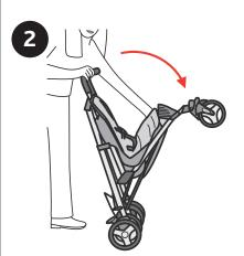
2. Release the side-mounted locking device and push the front part of the stroller forward.
