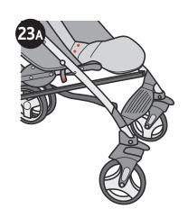
23A, 23B. Fasten the snaps (23A). Fit the fabric cover to the leg rest, then fasten the buckles (23B).
