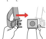
5. The Shoulder Strap Connector is designed to break away from the Waist Clip when not secured in the Crotch Strap Buckle.
