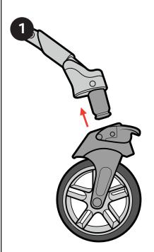
1. Attach the Front Wheel to the Stroller Frame by lining up and inserting the Front Wheel Post into the corresponding opening on the Front Wheel, as shown.
