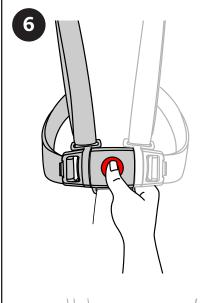
6. The safety harness can be released by pressing the button on the center of the Crotch Strap Buckle and pulling both Waist Clips out.
