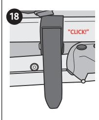
18. When the stroller is closed, the locking device located on the side of the stroller will automatically lock it in the close position, preventing it from accidentally opening.
