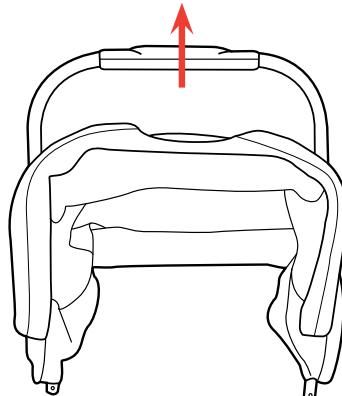
11. To remove the Bassinet Frame arms, lay the Bassinet Frame on its side. Locate the zippers on each side of the Bassinet Frame end, as shown. Undo both zippers and pull out the Bassinet Frame arm. Repeat for the other side and set both arms aside.
