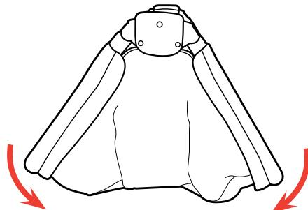
5. To Fold the bassinet, first remove the mattress. Then, press in on the Release Buttons on the Bassinet Hinge, as shown. The ends will fold down.
