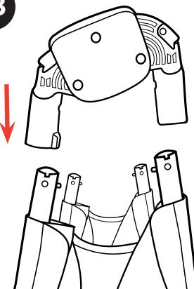
13. Line up the Bassinet Hinge end with the keyway to the Bassinet Frame arm with the pin and insert the arm into the Hinge. (See fig. A)
