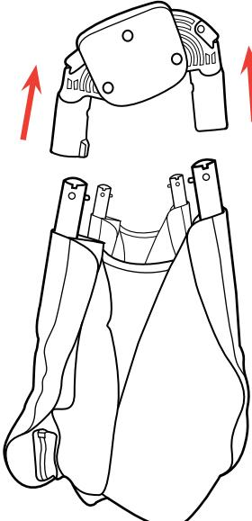
10. Remove the Bassinet Hinges from the Bassinet Frame. Locate 2 snap buttons on the Bassinet Hinge as shown. Press in on both snap buttons, one at a time, and pull up on the Bassinet Hinge to remove. Repeat for the other Bassinet Hinge.
