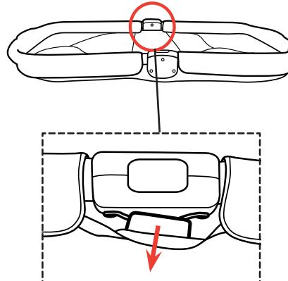
8. To remove the Bassinet Fabric from the Bassinet Frame, pull out the plastic tab from the metal bracket located on the side of the Bassinet Hinge. Repeat for the other side.
